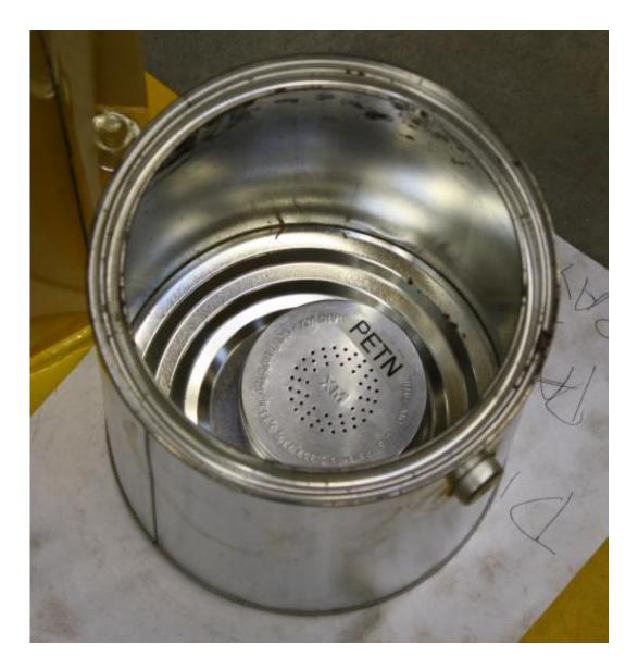
Test container of the NIST odor-releasing material hiding in a pail waiting to be discovered. Credit: Talbott/NIST
