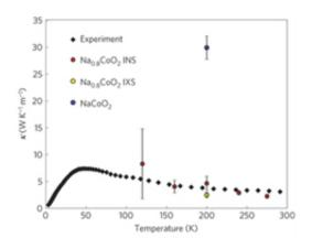
The measured thermal conductivity of  $Na_{0.8}CoO_2$  (black) well compare with the calculated lattice contribution to the thermal conductivity for the  $Na_{0.8}CoO_2$  superstructure comprising a square array of tri-vacancy clusters. Lattice contribution was obtained from the phonon lifetimes from neutrons (red) in a large temperature range and X-rays (yellow) at 200K. The calculated values for  $NaCoO_2$  (blue) are a factor of six higher.
