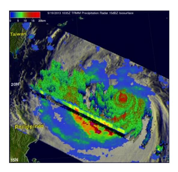
On Sept. 19 NASA's TRMM satellite saw rain falling at a rate of over 140mm/~5.5 inches (red) per hour in the powerful storms within Super Typhoon Usagi's eye wall. Credit: NASA/SSAI, Hal Pierce
