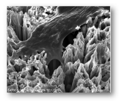
This is a bone cell anchoring itself to a surface of titanium dioxide nanotubes. Because osteoblasts readily adhere to this novel surface, dental implants coated with TiO2 nanotubes could significantly improve healing following dental implant surgery. Credit: Tolou Shokuhfar
