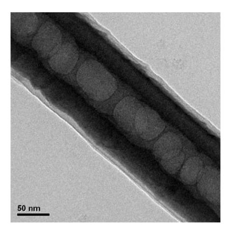
This cutaway view of a titanium dioxide nanotube reveals the drug sodium naproxen on the inside. On the surface of a dental implant, these nanotubes could release this anti-inflammatory drug or other pharmaceuticals that could speed healing. Credit: Tolou Shokuhfar
