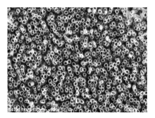
This shows a forest of titanium dioxide nanotubes etched into metallic titanium. The surface holds promise for improving the longevity of dental implants. Credit: Tolou Shokuhfar
