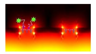
Localized surface plasmon resonance (bright areas) around a gold nanohole enhances the fluorescence of a biomarker dye (Y-shaped molecule) when a specific molecule of interest (purple circle) is present. Credit: 2013 A\*STAR Institute of High Performance Computing
