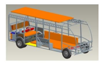
Modular batteries (orange) can be integrated easily in the free space of the vehicle. Credit: KIT
