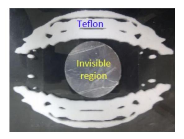
Device photo. The white 'eyelid' shaped cloak is made of Teflon which has permittivity about 2 near 15 GHz. The center invisible region is replaced by an aluminum disk of diameter =  $60 \text{ mm} = 3\lambda$ . The sample is 5 mm in thickness. In measurement there is no air gap between the sample surface and the measurement waveguide plates. Credit: arXiv:1308.6049 [physics.optics]
