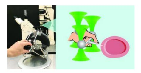
This is a conceptual representation of a highly nimble micromanipulation experimental setup. Cells can be explored with advanced laser trapped microtools that extend the operator's sense of touch thanks to a specifically designed haptic teleoperated optical tweezers. Credit: Pacore/UPMC
