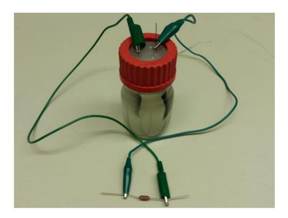
Stanford scientists have developed a "battery" that harnesses a special type of microbe to produce electricity by digesting the plant and animal waste dissolved in sewage. Credit: Xing Xie,Stanford Engineering
