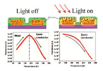
This image shows how electrons in the gold nanorods get excited when exposed to light, then are absorbed into a thin film of zinc oxide, changing the properties of the composite from a metal into a semiconductor. Credit: ACS Applied Materials & Interfaces. Credit: Washington University
