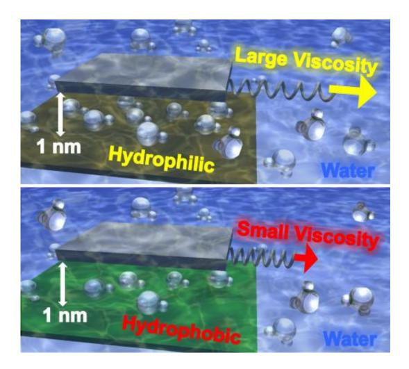
This illustration shows how the different effective viscosity of water affects the force required to slide two surfaces separated by a thin layer of water when confined by a hydrophilic material or a hydrophobic material. Credit: Elisa Riedo
