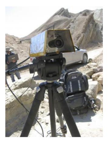
Scientists test TextureCam in the Mojave Desert in California. This advanced camera system for planetary rovers can scientifically assess images of rocks itself, whereas current rovers require scientists on Earth to do the analysis. Credit: Kiri Wagstaff
