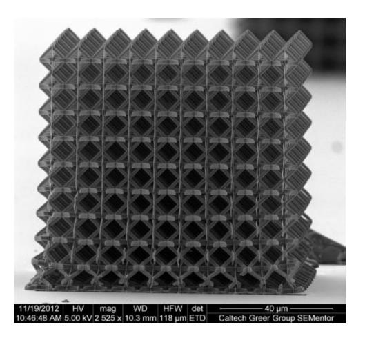
Three-dimensional, hollow titanium nitride nanotruss with tessellated octahedral geometry. Each unit cell is on the order of 10 microns, each strut length within the unit cell is about three to five microns, the diameter of each strut is less than one micron, and the thickness of titanium nitride is roughly 75 nanometers.
