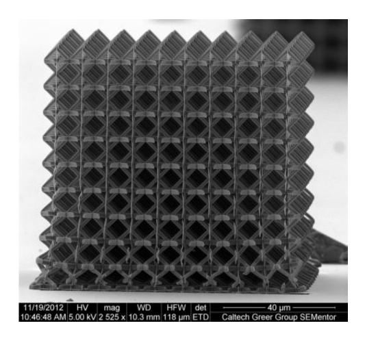
Three-dimensional, hollow titanium nitride nanotruss with tessellated octahedral geometry. Each unit cell is on the order of 10 microns, each strut length within the unit cell is about three to five microns, the diameter of each strut is less than one micron, and the thickness of titanium nitride is roughly 75 nanometers.
