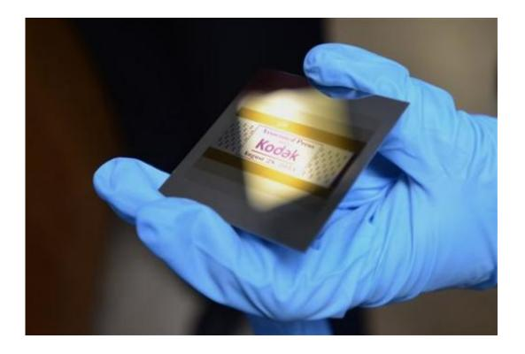
This Aug. 28, 2013 photo shows an example of what a piece of silicon looks like with Kodak print inhibiting ink at Kodak research labs in Rochester, N.Y. Kodak print inhibiting ink is used for printing electronics. (AP Photos/Heather Ainsworth)
