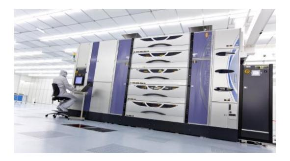
A technician sits at a track system at imec Belgium, an independent nanoelectronics microelectronics research center. The system coats, bakes and develops thin polymer films on silicon wafers, which are critical steps in the fabrication of samples that imec provides to Paul Nealey's research group at the University of Chicago's Institute for Molecular Engineering. Credit: Copyright imec
