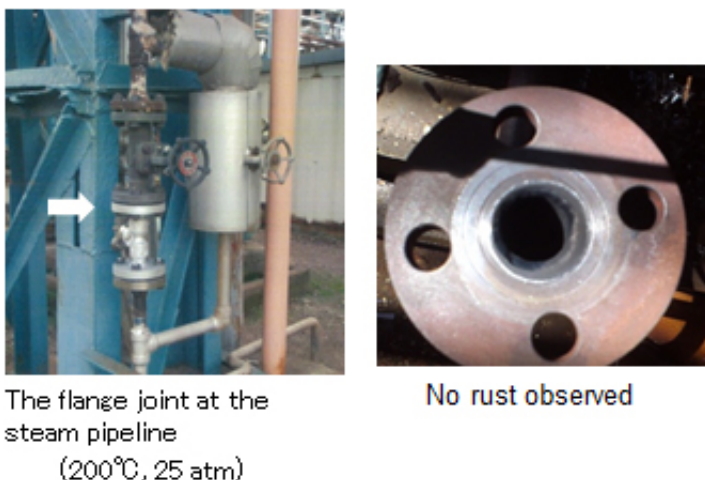
Figure 3: The location of the pipeline where the test was conducted (left) and flange surface after gasket removal (right). Credit: Befu Works of Sumitomo Seika
