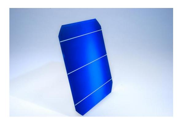
New large area cells (156x156mm2) achieve 20.5% average efficiency using Nickel/Copper plating on p-type Czochralski Silicon (Cz-Si) material.
