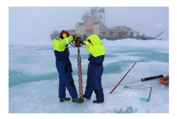
Researchers from the Oden Arctic Technology Research Cruise, coordinated by the Norwegian University of Science and Technology's Sustainable Arctic Marine and Coastal Technology research centre, drill an ice core on a floe off the northeast coast of Greenland. Credit: Taisiya Sinitsyna, NTNU
