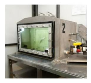
Hydraulic chambers will simulate extreme pressure changes to test the decompression limits fish can safely endure. The chambers are nominated for best new invention at the Engineers Australia Excellence Awards. Credit: Water Research Lab
