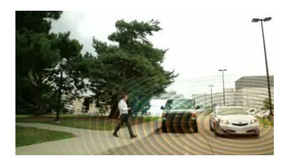
(Phys.org) —Honda Motor Company Ltd has posted a video on its website demonstrating new technology it's developing to help prevent cars from running into pedestrians. Based on already existing vehicle-to-vehicle (V2V) network technology, the system called by Honda an advanced vehicle-to-pedestrian (V2P) safety system aims to warn both drivers and pedestrians carrying smartphones of a possible collision.
