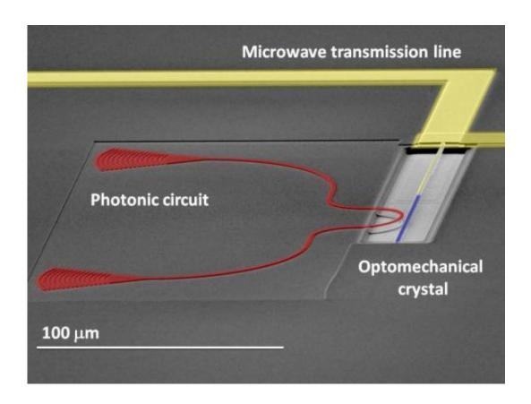
This is a schematic of electro-optomechanical transduction in the piezoelectric optomechanical crystal. Credit: Joerg Bochmann & Amit Vainsencher, UCSB
