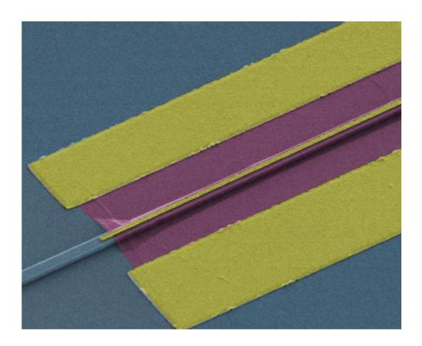
The light signal arrives throuth a waveguide (left), in the 2 micrometer wide graphene sheet, electrical current is generated.
