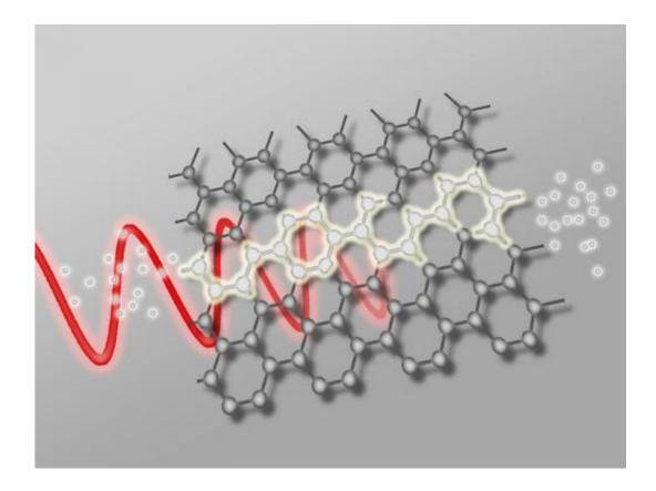
Graphene - a two dimensional sheet made of carbon atoms - can convert light into electrical current.
