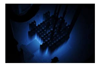
INL's NRAD reactor, shown here during operation, enables non-destructive examination of nuclear fuels and materials.
