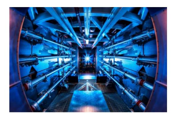
This image shows the preamplifiers of the National Ignition Facility. The unified lasers deliver 1.8 megajoules of energy and 500 terawatts of power -- 1,000 times more than the United States uses at any one moment. Credit: Damien Jemison/LLNL
