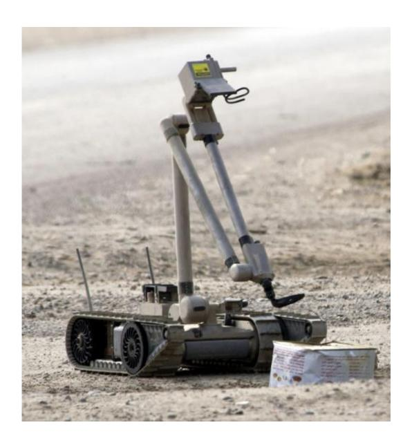
A United States Army explosive ordnance disposal robot pulls the wire of a suspected improvised explosive device in Iraq. Credit: U.S. Navy photo by
