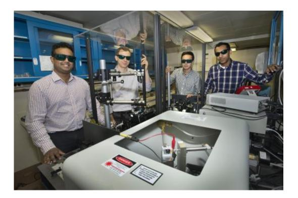
Nanditha Dissanayake, Matthew Eisaman, Yutong Pang, and Ahsan Ashraf display the setup used to track the flow of electrons through the photoactive layer of organic solar cells. The red and black wires in the box in the foreground (also shown in close-up) are connected to a solar cell that is in contact with a prism. The prism guides laser light through the cell in a range of specific directions to gain precise information about how electrons flow.
