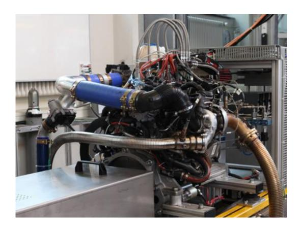
ETH researchers redesigned the conventional diesel engine of a VW Golf to run on 90% natural gas. Credit: Tobias Ott / ETH Zurich
