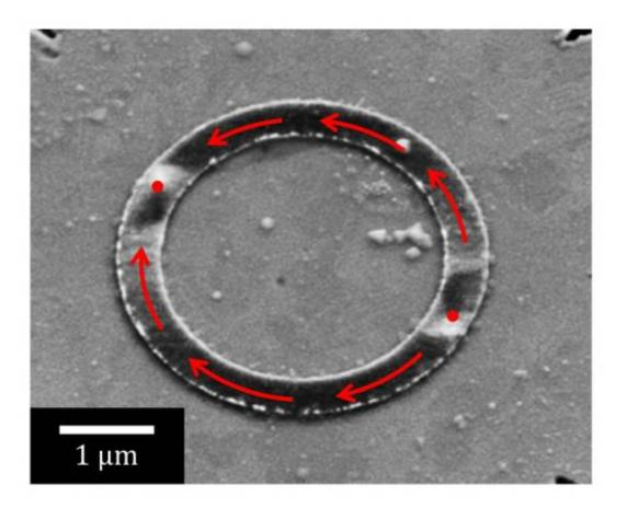
This is an image of a ferromagnetic ring prepared using a scanning electron microscope: The magnetization (black/white contrast) runs along the ring and forms two domain walls. Credit: André Bisig, Institute of Physics, Johannes Gutenberg University Mainz
