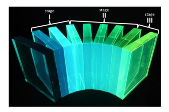
The concentration of fluorescent benzoxanthene (Y11) increases in a plastic from left to right, with the sample at the far left being pure plastic with no added molecules. In each sample, ultraviolet light is absorbed and light ranging from blue to green is emitted as a function of the benzoxanthene concentration.
