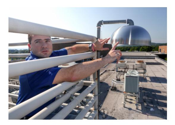
Dr. Phillip Bitzer, an assistant professor of atmospheric science, has installed a lightning sensor on the roof of UAH's National Space Science Technology Center. A still camera is being installed to provide time-lapse photos of weather that will be viewable on the web. Dr. Bitzer also plans to install two high-speed video cameras in this location as well. Credit: Mike Mercier | UAH
