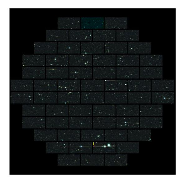
Composite Dark Energy Camera image of one of the sky regions that the collaboration will use to study supernovae, exploding stars that will help uncover the nature of dark energy. The outlines of each of the 62 Charged Coupled Devices can be seen. This picture spans 2 degrees across on the sky and contains 520 megapixels.
