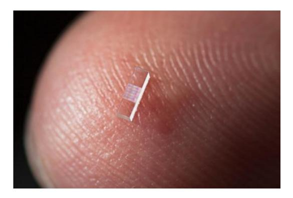
The key to the accelerator chips is tiny, precisely spaced ridges, which cause the iridescence seen in this close-up photo. Credit: Matt Beardsley, SLAC National Accelerator Laboratory
