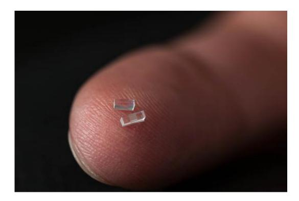
SLAC and Stanford scientists used nanofabricated chips of fused silica just three millimeters long to accelerate electrons at a rate 10 times higher than conventional particle accelerator technology. Credit: Matt Beardsley, SLAC National Accelerator Laboratory
