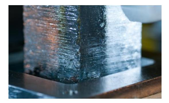
This image shows an ice core sample melting on a continuous system inside the ultra-trace ice core analytical laboratory at the Desert Research Institute in Reno, Nevada. Credit: Desert Research Institute - Sylvain Masclin
