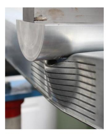
This crash test is designed to establish how much a sample component deforms under a defined bending stress. Credit: Fraunhofer IWS
