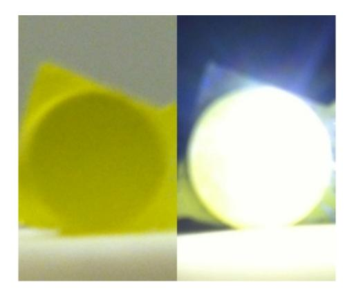
This is a photograph of bright white light (right) achieved using lasers in combination with phosphors next to an image of the phosphor with no illumination. Credit: K.Denault/UCSB
