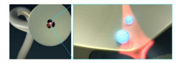
The micro-structured optical fibre has been employed as a nanoliter-volume spectroscope to analyse the optical properties of nanocrystals. Credit: Matthew Henderson
