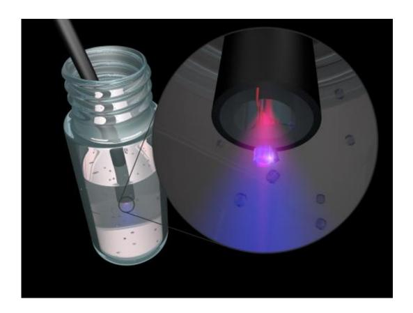
The super-sensitive nanocrystals enable the micro-structured optical fibre to detect and track the movement of a single nanocrystal remotely. Credit: Dr Mathieu Juan
