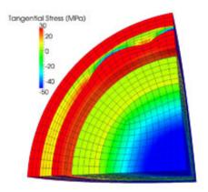
A simulation using BISON shows how a defect in a TRISO nuclear fuel particle can impact the surrounding containment layers during reactor operation.
