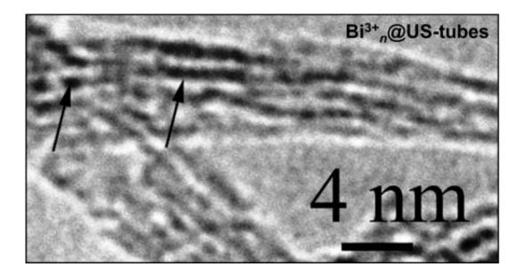
An electron microscope image shows bismuth ions (dark lines) sitting inside carbon nanotubes. The material created at Rice University is a contrast agent that may allow clinicians to track the progress of stem cells in the body with a CT scanner. Credit: Eladio Rivera/Rice University
