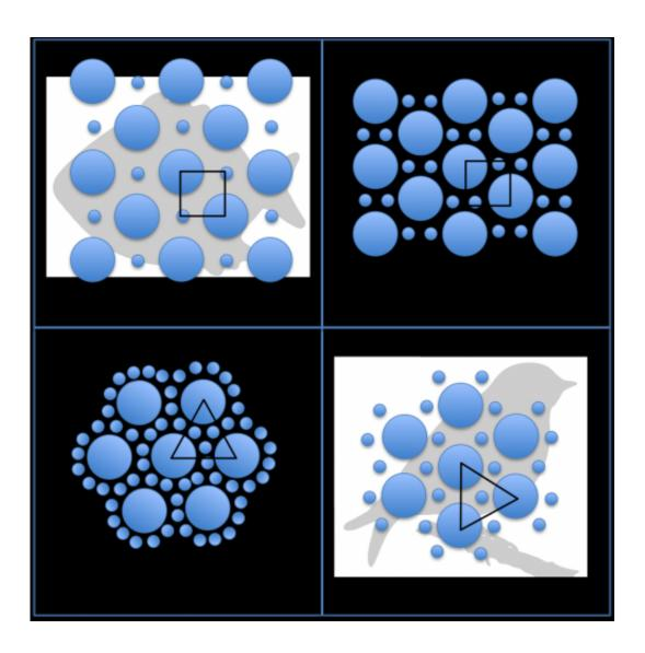
Inspired by how blood vessels are packed in the avian lung and the fish swim bladder, scientists have found the best way to pack tubes in a carbon dioxide capture unit. Credit: ThinkStock/XiaoZhi Lim
