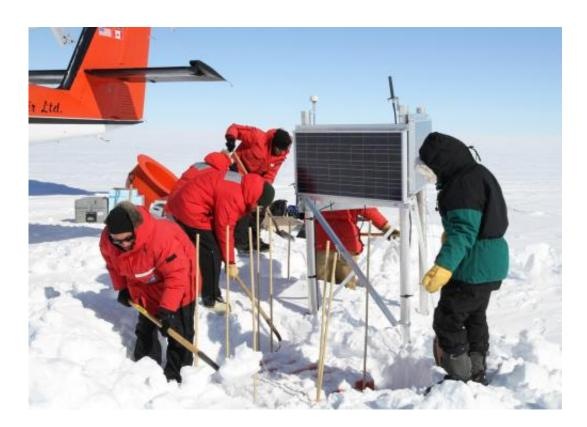
The POLENET team buries a seismic station in Antarctica. The tall poles and solar array will help the next team find the station. The orange box holds batteries and the electronic equipment for the instrument. Wiens, shovel in hand, is to the left. Credit: Rachel Gesserman
