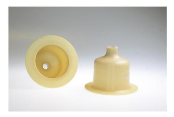
The test piece's special shape permits substantially more realistic testing scenarios for plastic components. Credit: Fraunhofer LBF
