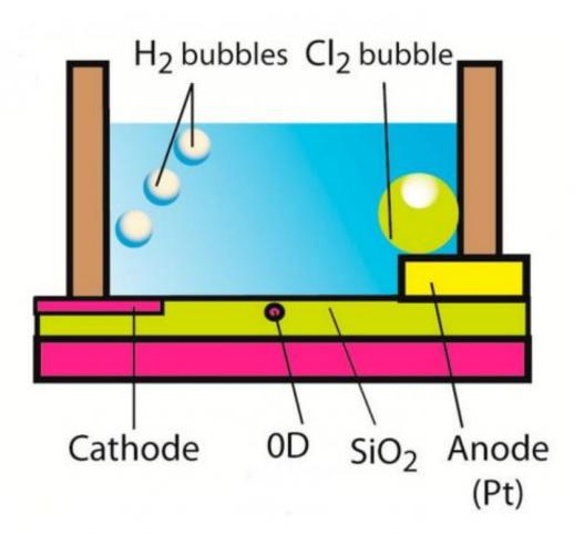
A zero-dimensional transistor is placed in contact with a water droplet containing NaCl ions. A current between the anode and cathode generates hydrogen and chlorine bubbles, which the transistor can detect and transform into electric pulses. Credit: N. Clément, et al. ©2013 American Chemical Society
