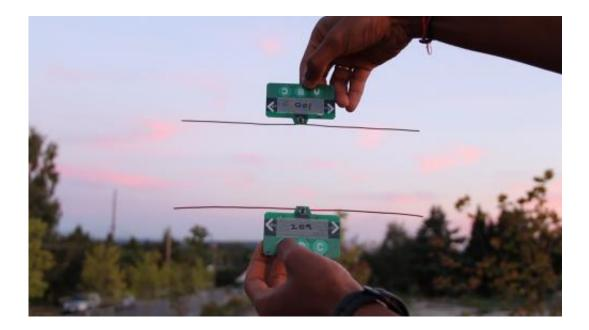
Researchers demonstrate how one payment card can transfer funds to another card by leveraging the existing wireless signals around them. Ambient RF signals are both the power source and the communication medium. Credit: University of Washington
