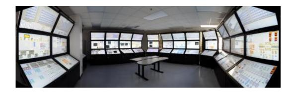
The Department of Energy's new Human System Simulation Laboratory at Idaho National Laboratory is a full-scale virtual nuclear control room that can test the safety and reliability of proposed technology replacements before they are implemented in commercial nuclear control rooms. Credit: Idaho National Laboratory
