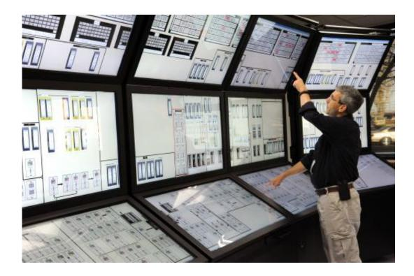
The Department of Energy's new Human System Simulation Laboratory at Idaho National Laboratory is a full-scale virtual nuclear control room that can test the safety and reliability of proposed technology replacements before they are implemented in commercial nuclear control rooms. Credit: Idaho National Laboratory
