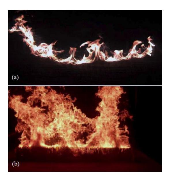
Photos taken inside the wind tunnel show the "peak and valley" structure of flames, looking upwind. In the top image, flames are approximately 0.15 meters (6 inches) tall. In the bottom image, flames approximately 2 meters (6.5 feet)
