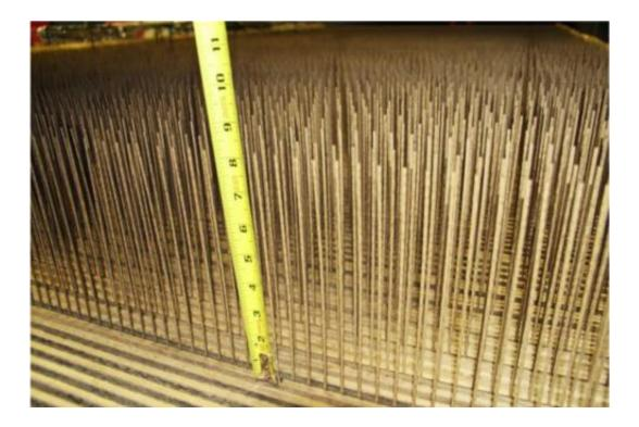
The model fuel bed, made up of laser-cut cardboard strips arranged in rows of "combs."
