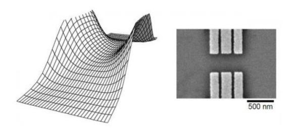
Left: Electrons moving through a short, narrow nano wire experience this as a trip through a mountain pass. Right: Electron microscope image of the device with an adjustable nano wire. Electrons move from left to right under the surface of a semiconductor (dark). The precise shape of the nano channel can be set by applying an electrical voltage to the electrodes on the surface.
