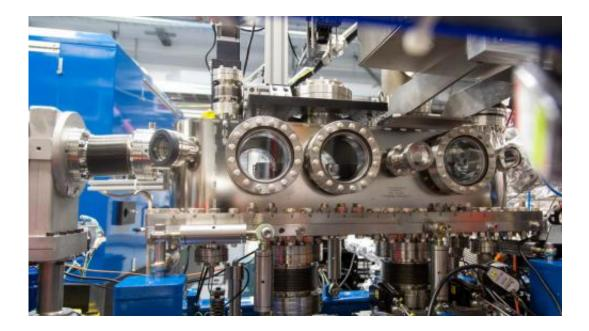
This soft X-ray split-and-delay system divides individual X-ray laser pulses into two separate, closely spaced pulses at SLAC's LCLS. Credit: Matt Beardsley/SLAC
