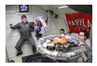
In the spring of 2013, RINGS was tested for the first time in a microgravity environment on NASA's reduced gravity aircraft. UMD graduate students Allison Porter and Dustin Alinger were on hand to
