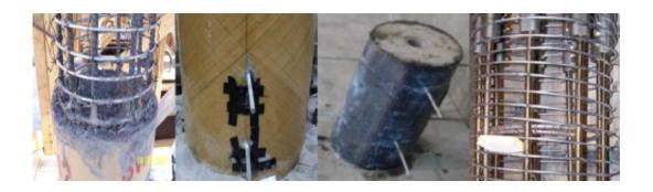
Traditional bridge columns are constructed from concrete and reinforced steel, which are seldom effective against earthquakes. But new research suggests that replacing concrete and steel with smart materials is a good alternative. From left: cement-polyvinyl fiber mixture; fiberglass column; carbon fiber column; nickel titanium shape memory alloy, or nitinol. Credit: Dr. M. Saiid Saiidi, NEES@University of Nevada, Reno
