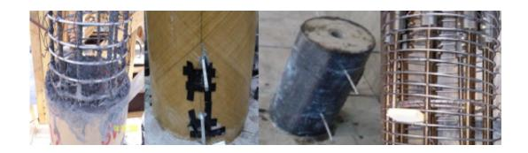
Traditional bridge columns are constructed from concrete and reinforced steel, which are seldom effective against earthquakes. But new research suggests that replacing concrete and steel with smart materials is a good alternative. From left: cement-polyvinyl fiber mixture; fiberglass column; carbon fiber column; nickel titanium shape memory alloy, or nitinol. Credit: Dr. M. Saiid Saiidi, NEES@University of Nevada, Reno
