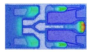
The triangular mesh used to model the properties of a hard disk read/write head. The colors represent the pressure profile of the head; red indicates areas of high pressure. Credit: A\*STAR Data Storage Institute
